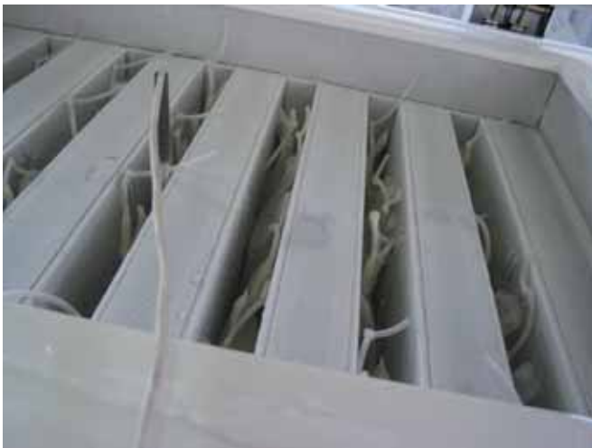
Internal case of the rapid freezer with standard 450 ml. bags in freezing
